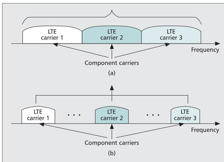
**Figure 1.** Carrier aggregation types: a) continuous; b) non-continuous.
